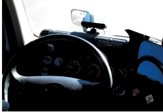
Figure 5. Photo. Installation position for Smart Eye.
